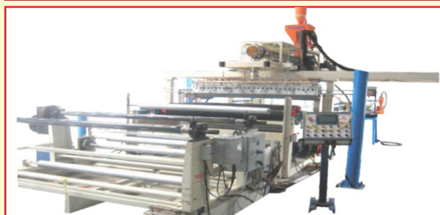
Extrusion Lamination Plant for Woven Sacks
