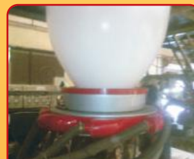
VI-A ABA L/D Plant Rotating Air Ring With Irish Ring Assembly
