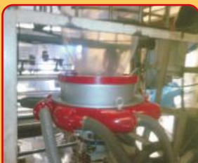
VI-A Rotating Air Ring with Irish Ring Assembly L/D Shreenk Film
