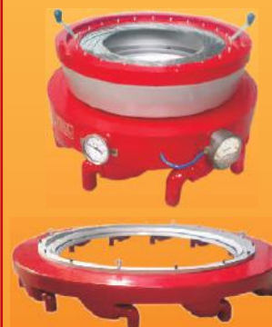
Air Ring For Tarpaulin Plant wide width film up to 6 meter
