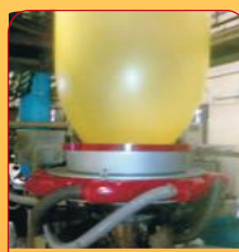
VI-A Rotating Air Ring with Irish Ring Assembly L/D Stretch Film
