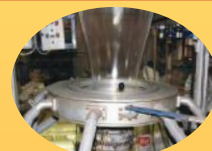
Air Ring For L/D & L.L.D.PE
