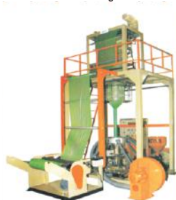
Two Layer with Optional Rotating Die
