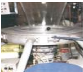
Dual Lips Rotating Air Ring For L.L.D. Higher Output Rates, Clarity & Without Gauge Variation
