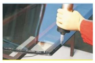
Windshield bonding: GENIOSIL® XT silane-modified polymers from Munich-based chemical group WACKER make it possible to formulate strong but highly elastic adhesives of the kind needed for direct glazing.
